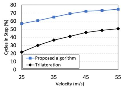
Fig. 12: Simulation cycles percentage during which the UAV stays in step versus the UAV velocity.
