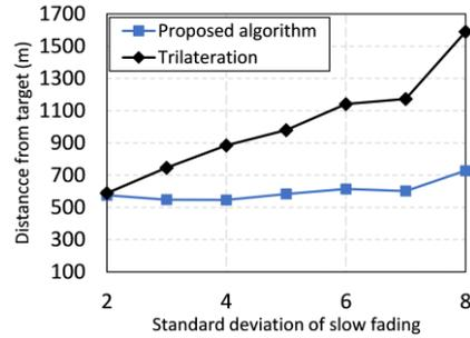
Fig. 6: Average distance between the UAV and the target versus  $\sigma$ .
