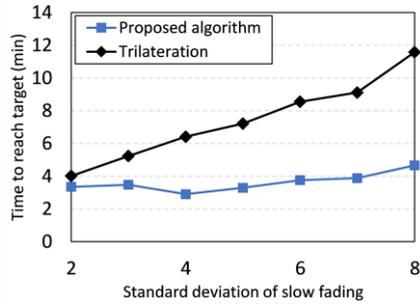
Fig. 5: Minimum elapsed time until the UAV reaches the target versus  $\sigma$ .
