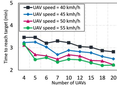
Fig. 14: Minimum elapsed time until the UAV reaches the target versus the size of the swarm, for different UAV speeds.
