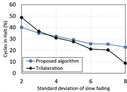
Fig. 7: Simulation cycles percentage during which the UAV stays in halt versus  $\sigma$ .
