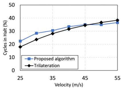
Fig. 11: Simulation cycles percentage during which the UAV stays in halt versus the UAV velocity.
