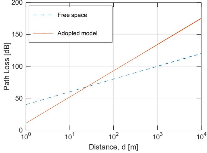
215 Fig. 1: Comparison of the free-space and the adopted RF model. The dashed line represents the path loss according to the free-space propagation scheme. The solid line depicts the path loss according to the adopted RF model.
