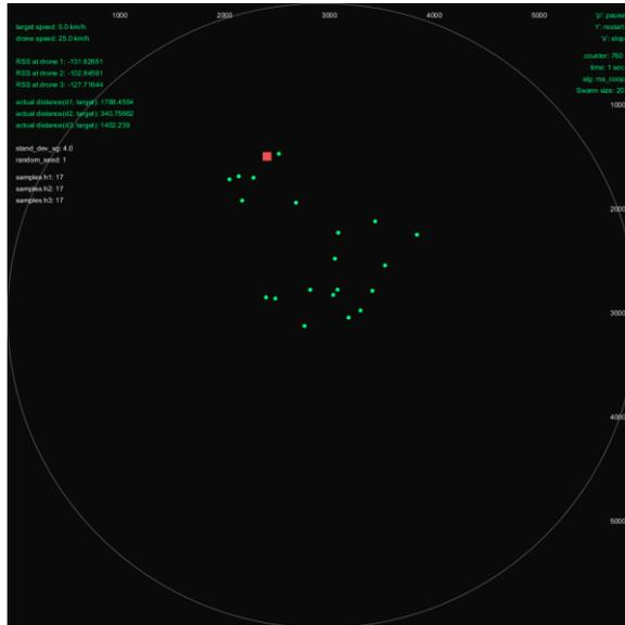
380 Fig. 3: Visual representation of a devised simulated environment. The square represents the target and the dots represent the UAVs.
