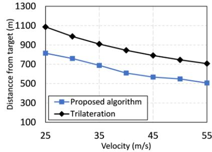
Fig. 10: Average distance between the UAV and the target versus the UAV velocity.
