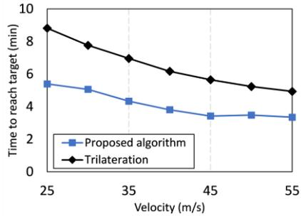
Fig. 9: Minimum elapsed time until the UAV reaches the target versus the UAV velocity.
