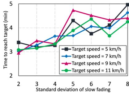
Fig. 13: Minimum elapsed time until the UAV reaches the target versus  $\sigma$ , for different target speeds.
