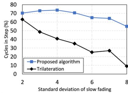
Fig. 8: Simulation cycles percentage during which the UAV stays in step versus  $\sigma$ .
